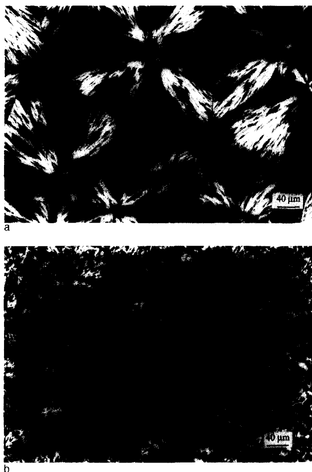
Figure 3 Polarized light microscope photographs of PCL (a), and PCL-PTMC (b), crystallized at 46^\circ\text{C}
